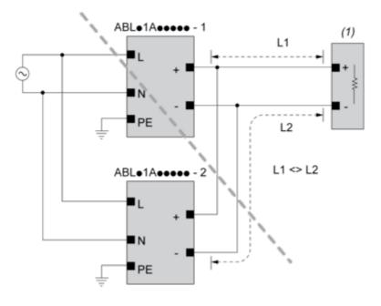
(1): Load ABLx1Axxxxx-1 = ABLx1Axxxxx-2 max 2 x ABLx1Axxxxx L1 = L2  $\Delta V max 25 mV$   $I_{Load} < 90\% 2 x I_{nom}$
